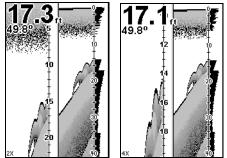
Split Zoom Sonar Chart. First image (left) shows the left window zoomed to 2X. The second image (right) shows the left window zoomed to 4X. The depth overlay data is set to the default large text size. The water temperature is set to the medium text size.
